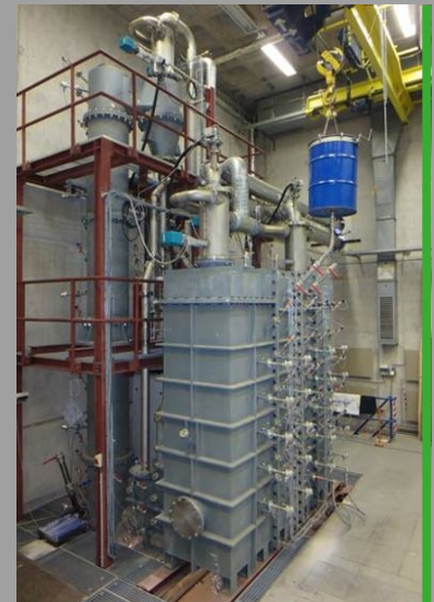
ANICA 300 kW th pilot plant at TU Darmstadt.
